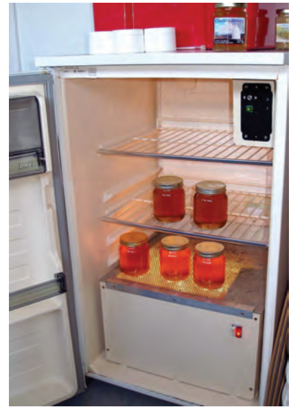
My honey warmer, made from an old fridge and a couple of light bulbs.
